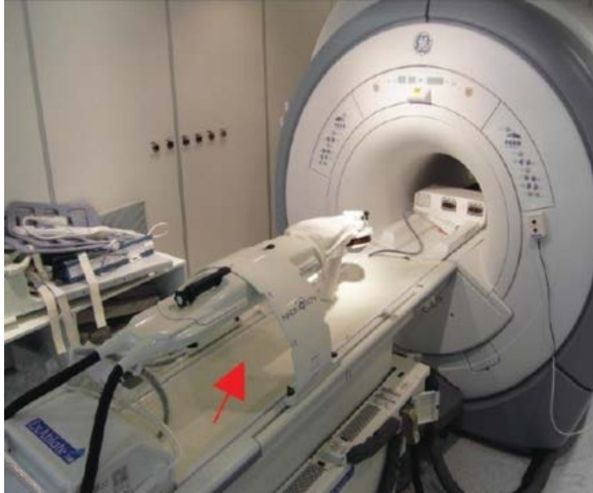
Fig. 1-3: MRI-guided surgical application of the Innomotion robotic system (red arrow). It has pneumatically actuated 5 DOF and manually actuated 2 DOF [18].
